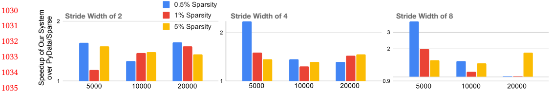
Fig. 28. Various stride length slicing operations across different square matrix sizes, parameterized by sparsity and plotted on a log-scale.
